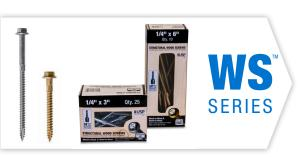
The **WS Wood Screw<sup>TM</sup>** is a self-drilling screw used for numerous framing applications. This screw features a reverse locking serration on the bottom of the screw head to help prevent over tightening against a steel plate. The USP head stamp identifies screws for easy inspection.
